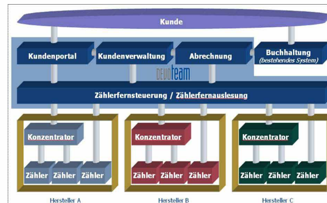
Devoteam BSS Automatic Meter Architecture
