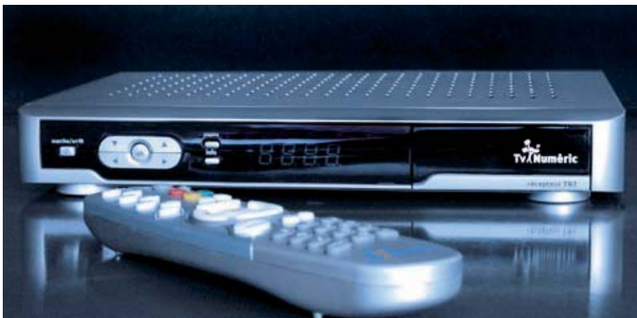
Set top box: Decoder for signals that are received via the house antenna.
